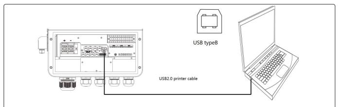
The user can read and modify device parameters through this port by using the host software. Please contact us for the host software installation package if you require one.
