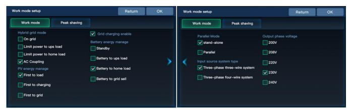
Home Load: connected to the GRID port of the machine, requires external CT for monitoring. UPS Load: connected to the LOAD port of the machine.
